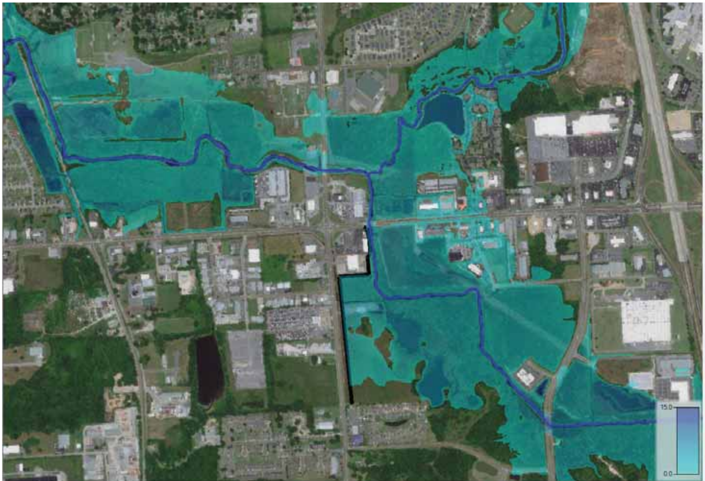
Figure 76. 0.10 AEP Levee Alternative Inundation Depth Map-Bullfrog Corner
